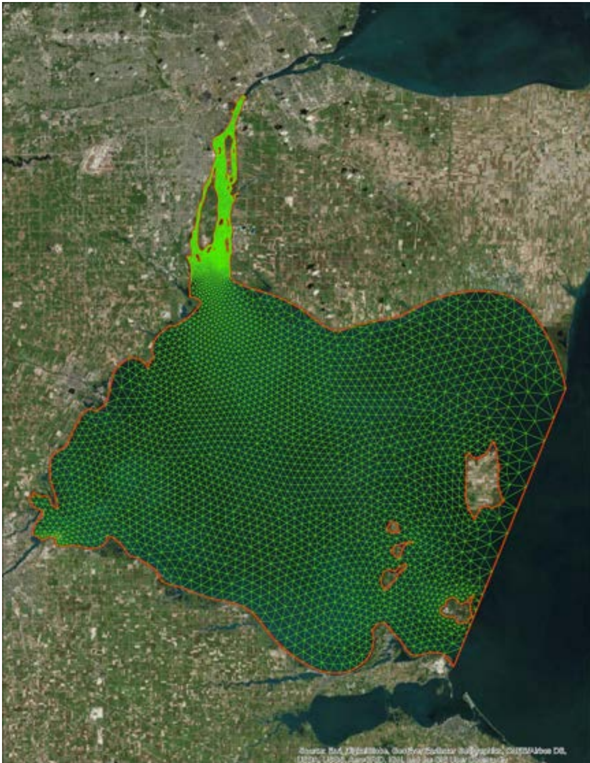
Figure 5: Wind-driven wave model (SWAN) mesh domain.
