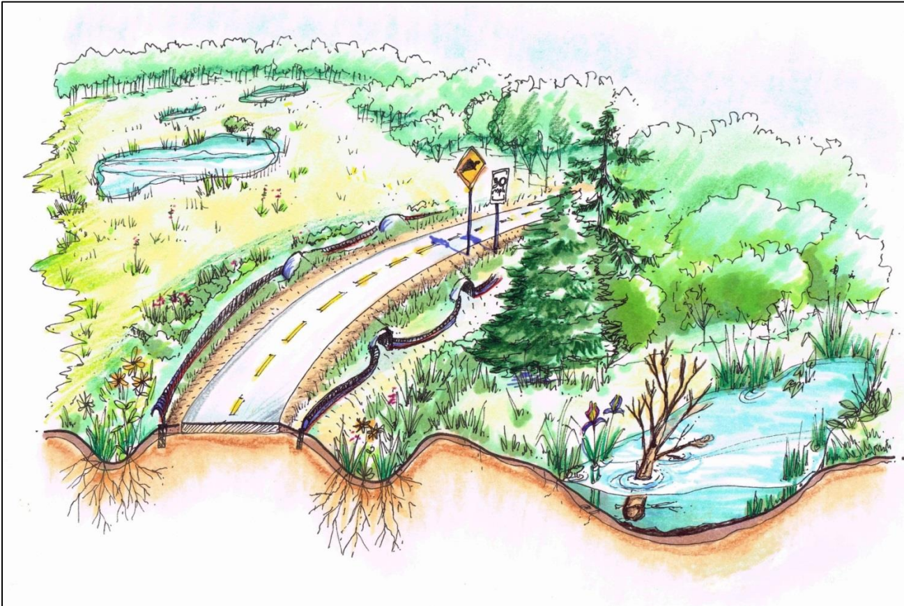
Figure 1. Conceptual drawing depicting a landscape modified to incorporate low or non-existent curbs, crossing structures and associated barrier fencing, reduced mowing, and wildlife crossing signs. Figure source: Michigan Amphibian and Reptile Best Management Practices manual (Mifsud 2014).
